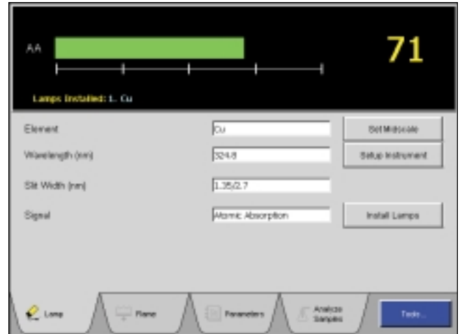
Lamp set up page automatically sets up the instrument when using a coded Lumina lamp.
